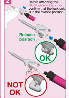
Place GC Push and Click Tip lightly on the syringe nozzle and push the lock unit down to the fixing position until you hear a click. Click by pushing Click **Fixing** position
